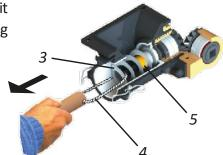
**03** - After cleaning, replace the endless spring (3), together with the locking ring (5), through the fixing tube (4), making sure that the endless spring (3) and the locking ring (5) are well positioned at the base of the shaft (6).
