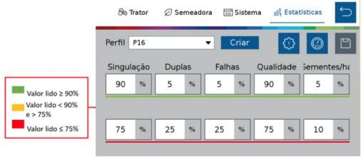
Configuration of statistics alarm parameters
