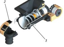
02 - Then, introduce the maintenance tube (3) in rotating movements to move the fertilizer to the bottom of the feeder. Then perform the necessary maintenance.
