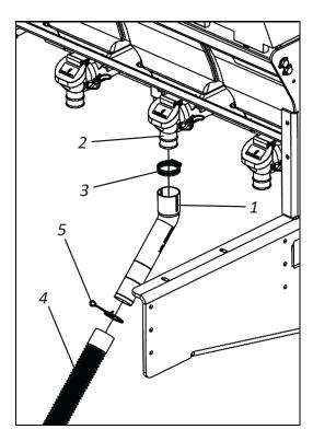
The Fertisystem system has safety outputs that guarantee the proper functioning of the system without damaging it. In case of clogging of the hose and the batcher, clean the batcher until the end of the hose near the furrower rod
