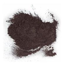
The graphite is essential for the system to work and also for perfect seed distribution, reducing doubles and failures, broken seeds, and system wear.
