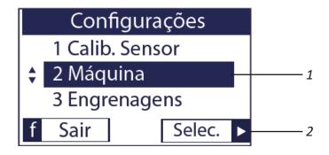
In the machine configuration (1), click 'Select  $\triangleright$  (2) to enter the number of Rows using the buttons  $\spadesuit$  (3).
