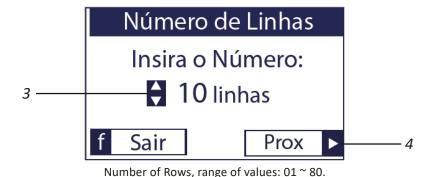
After selecting the number of Rows contained in the machine, press the 'Next' key  $\blacktriangleright$  (4) to select the Row spacing using the buttons  $\spadesuit$  (5).
