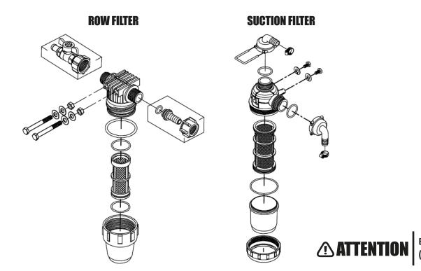
Before starting cleaning the suction (1) and Row (2) filters, wear PPE equipment (especially gloves). Ignoring this warning can cause serious illness or even death.
