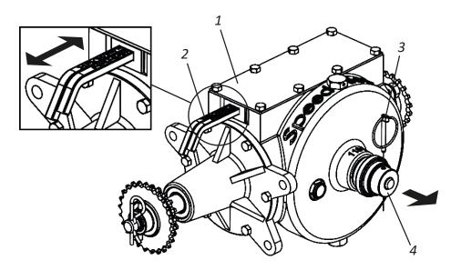
**02** - To move the levers, remove the lock (3), pull the handle (4), then adjust the levers according to the example above. When combining is complete, return the handle (4) and replace the lock (3).
