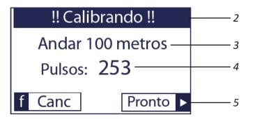
When starting the sensor calibration (2), the machine must be moved for exactly 100 meters (3) and stopped.
