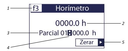
The F3 screen (1) indicates the total number of hours (2) of work with the ETD in three partials (3), which can be related to the keys  $\stackrel{\blacktriangle}{=}$  (4)
