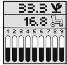
The operator can use usar to manually select which Row to monitor. Automatic counting will restart in 10 seconds after manual selection.
