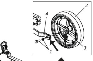
01 - Loosen the screws and washers (1), remove the wheel (2), adjust the wheel adjustment point (3) on the wheel support shaft adjustment (4), then secure the wheel (2) again with the washers and screws (1).
