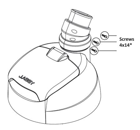
Position the new nozzle and insert the three 4x14 Phillips screws (removed from the old nozzle).
