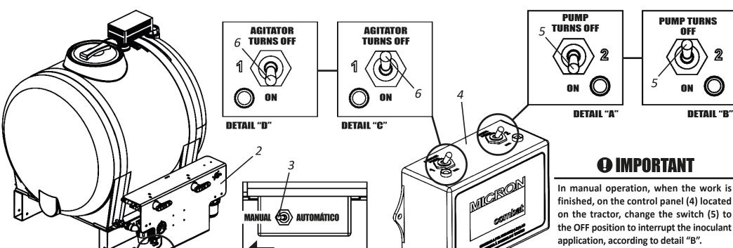
In manual operation, the inoculant application will not start the moment the DEMETRA is lowered, but the moment the switch (5) of the control panel (4) located on the TRACTOR is turned to the ON position.
