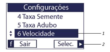
By clicking on 'Select.' (2) in the 'Speed' setting (1) it will be shown for how many hours (4) the machine has been working above the limit speed (3).
