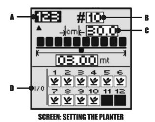
, select a planter configuration number using 01 - In field A press confirm by pressing again;
