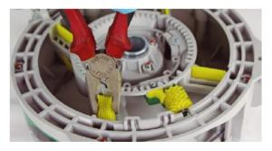
02 - With pliers, fit the ANTI SKIP inside the base and pull until fully fit.
