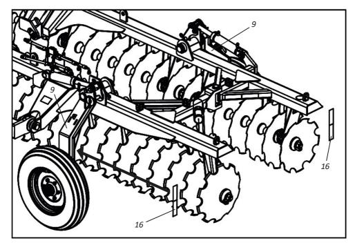
To attach the signaling stickers (16) correctly, lower the wheel axle supports (9) as shown above.
