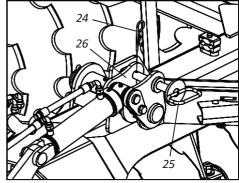
11 - Then, activate the hydraulic cylinder (26) to lower the tire (27) to the ground.
