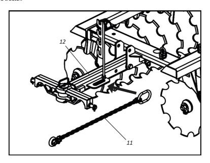
**06** - Then unlock the transport head (12) of point "A" through the lock (13), flat washer (14), remove the pin (15).
