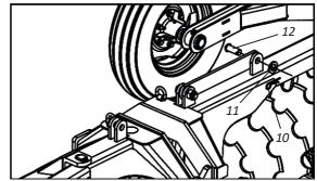
05 - Then, articulate the bar (13) by locking it in the frame (14) through the same pin (12), flat washer (11) and lock (10).
