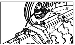
11 - Then, slowly approach the tractor to the NVF-T in reverse gear, paying attention to the application of the brakes at a distance of 3 meters from the NVF-T. Then, turn off the tractor engine, relieve the pressure of the control by pushing the lever a few times and check that the couplings are clean if not so, clean them.
