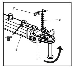
**08** - Then, level the coupling head (4) with the tractor's coupling through the hydraulic cylinder (5).
