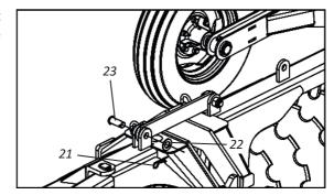
10- Then, articulate the bar (24), unlocking the frames and fastening it through the pin (23), flat washer (22), and lock (21).
