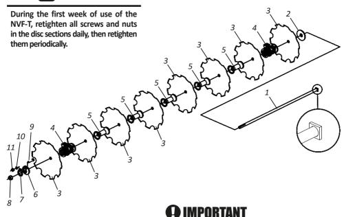
Check pages 22 to 25 for the correct mounting position of the disk sections (conventional system) on the front and rear frames.
