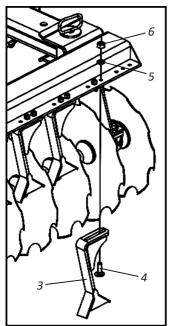
01 - From the tip to the center of the front (1) and rear (2) frames, secure the wipers (3) using screws (4), pressure washers (5) and nuts (6).
