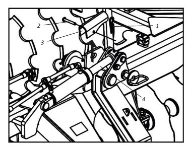
02 - Then, fasten the lock (3) to the wheel axle support (5), through the pin (2), and lock (1).
