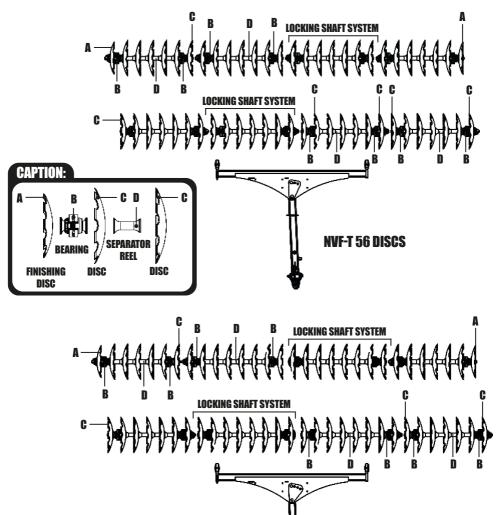
The disk sections (locking shaft system) are mounted only in the center of the NVF-T Front Right and Rear Left frames.
