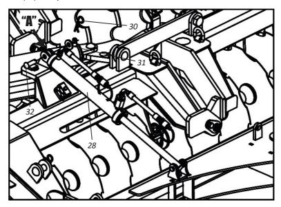
**15**- Then, through the coupling support (33) spin the hydraulic cylinder (28) to couple it to point "B" fastening through pin (32), flat washer (33), and lock (34).
