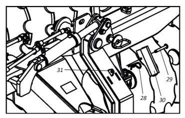
13- Then, couple the lock (30) to the hydraulic cylinder rod (32), fastening with the pin (29), and lock (28).
