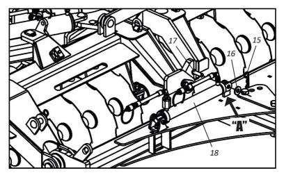
**07** - Then, through the coupling support (19) spin the hydraulic cylinder (18) to couple it to point "B" fastening through pin (17), flat washer (16), and lock (15).
