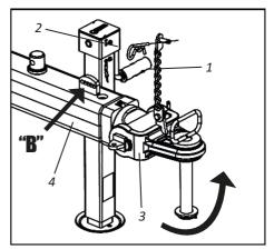
O4 - Then, level the coupling head (4) with the tractor's coupling using the adjuster (5).
