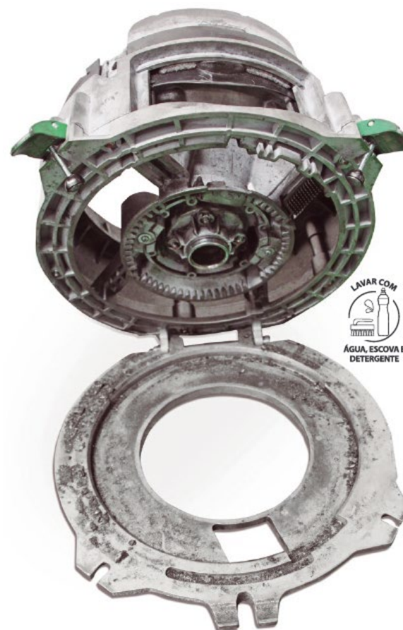
Counter-base of the TITANIUM batcher dirty with graphite.
