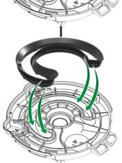
02 - Firstly, assemble the ends of the new seal on the metering cover.
