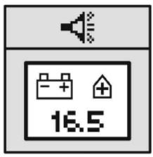
**SCREEN: SELF-TEST FAILURE**
