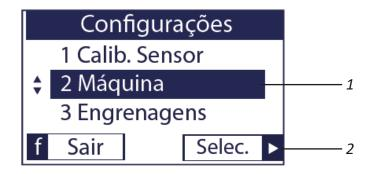
In the machine configuration (1), click 'Select  $\triangleright$  (2) to enter the number of Rows using the buttons  $\stackrel{\blacktriangle}{=}$  (3).
