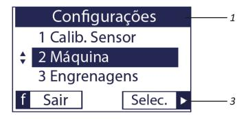
In the machine configuration (1), click 'Select'  $\triangleright$  (2) to enter the number of Rows using the buttons  $\stackrel{\triangle}{\bullet}$  (3).
