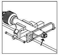
Cut the inner bars of the cardan in the same length as the protective tubes.
