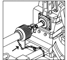
Do not connect the cardan chains while they are stretched. Keep a gap in the installation and consider angular movements.
