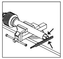
Remove all burrs and edges. Clean and grease the cardan bars.
