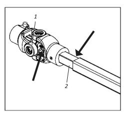
Lubricate the crossbars (1) with grease every 8 hours. The telescopic axle (2) must be lubricated weekly.
