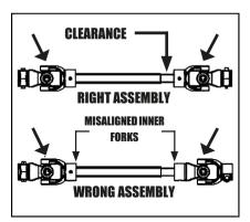
When assembling, observe that the internal and external terminals are always in the same plane, aligned. Also check the clearance on the telescopic axle, which should be of 5 to 7 cm.
