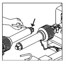
Secure the shaft halves from the shaft close to each other in the working position and mark the part to be cut.
