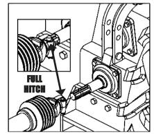
Attach the flange to TDP shaft of the tractor observing that the engagement will only be completed when lock (1) springs out.
