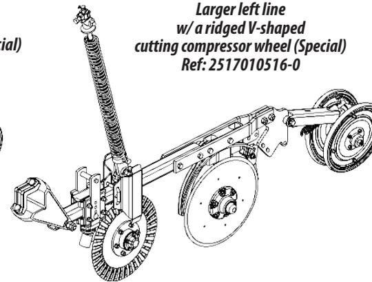
*Larger left line w/ a ridged V-shaped cutting compressor wheel (Special)
