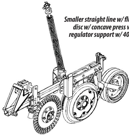
*Smaller straight line w/ fluted cutting disc w/ concave press wheel w/ regulator support w/ 40 mm bead*
