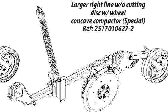
*Larger right line w/o cutting disc w/ wheel concave compactor (Special)
