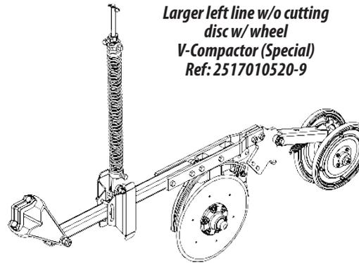
*Larger left line w/o cutting disc w/ wheel V-Compactor (Special)
