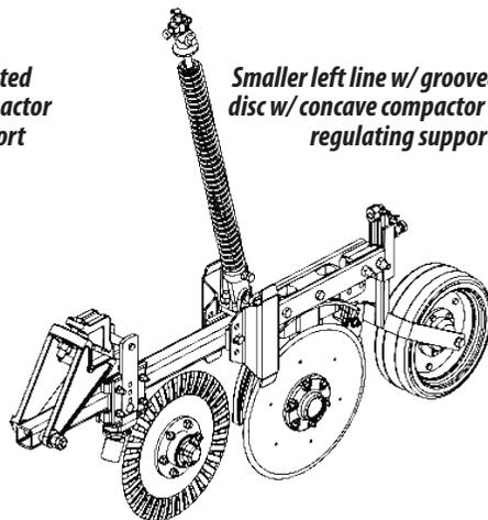
*Larger left line w/ grooved cutting disc w/ concave compactor wheel w/ regulating support*
