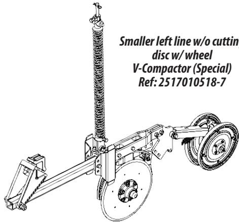
*Smaller left line w/o cutting disc w/ wheel V-Compactor (Special)
