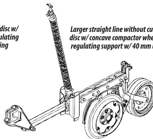
*Larger left line w/ cutting disc w/ concave press wheel w/ regulating support w/ 40 mm bead*
