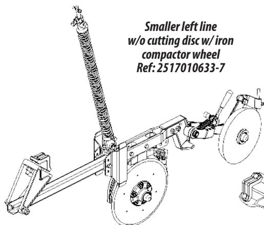
*Smaller left line w/o cutting disc w/ iron compactor wheel
