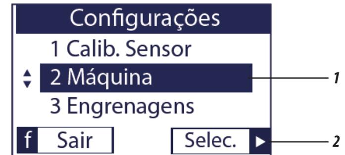
In the machine configuration (1), click on 'Selec.' (2) to inform the number of lines using the buttons ▲▼ (3).
