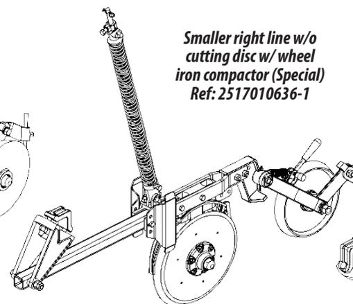
*Smaller right line w/o cutting disc w/ wheel iron compactor (Special)
