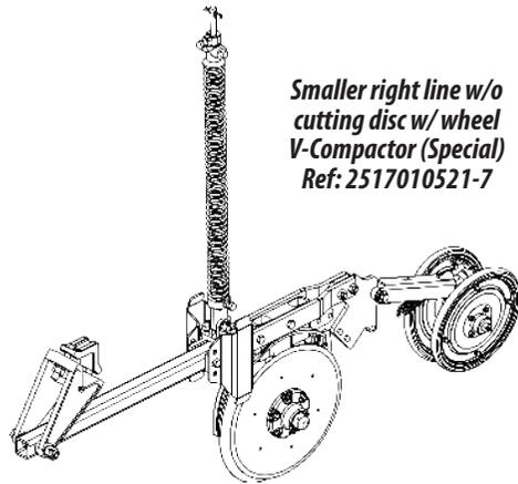
*Smaller right line w/o cutting disc w/ wheel V-Compactor (Special)
