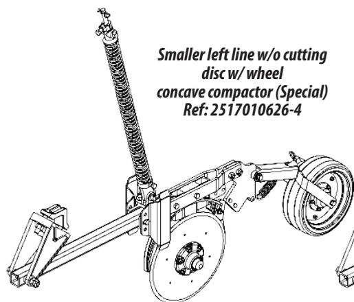
*Smaller left line w/o cutting disc w/ wheel concave compactor (Special)
