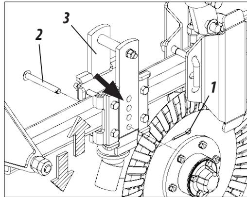
To move the ridged or plain cutting disc (1) in the horizontal position, proceed as follows:
