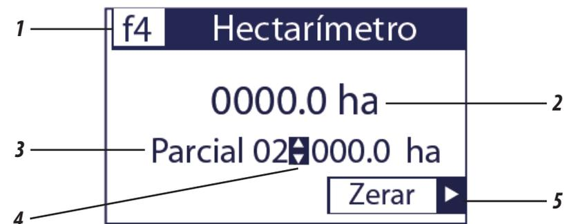
Screen F4 (1) indicates the total number of hectares worked (2) with the ETD, also in 3 partial ones (3), which can be selected using the keys
