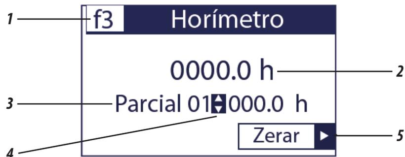
The F3 screen (1) indicates the total number of hours (2) of work with the ETD in three partials (3), which can be related to the keys
