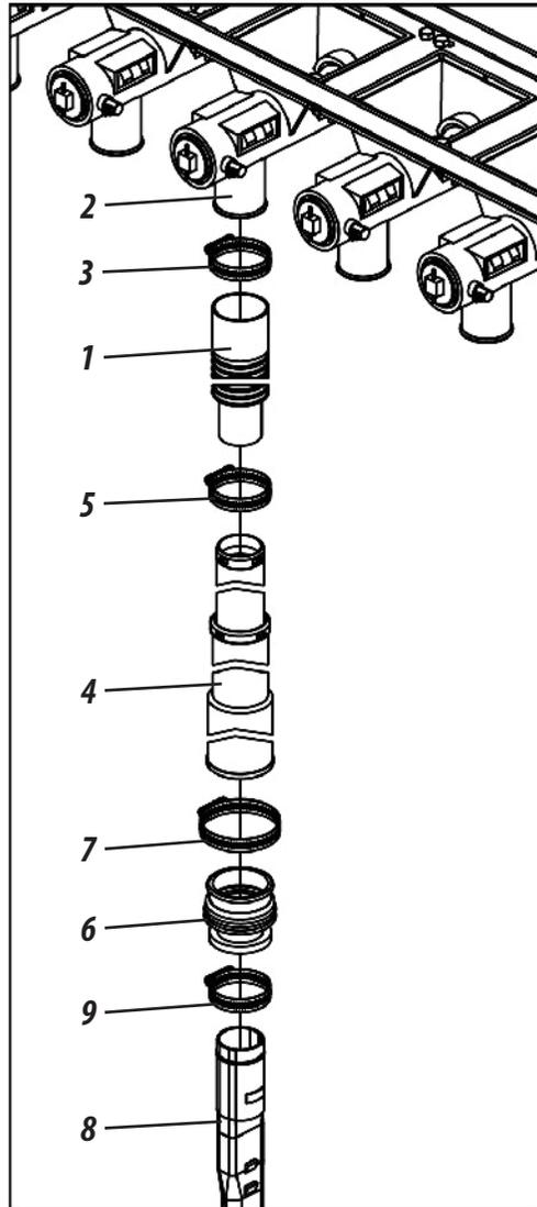
To send the fertilizer from the distributor to the ground, fit the hose (1) to the outputs of the independent conductor (2) through the clips (3). Then, attach the telescopic cable (4) to the hose (1) by attaching it through the clamp (5). Then, attach the rubber coupling (6) to the telescopic cable (4) by attaching it through the clip (7). Finish by attaching the spout (8) to the rubber coupling (6) by attaching through the clip (9).
