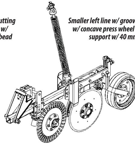
*Smaller left line w/ grooved cutting disc w/ concave press wheel w/ regulator support w/ 40 mm bead*
