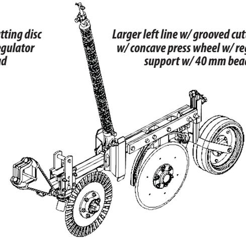
*Larger left line w/ grooved cutting disc w/ concave press wheel w/ regulator support w/ 40 mm bead*
