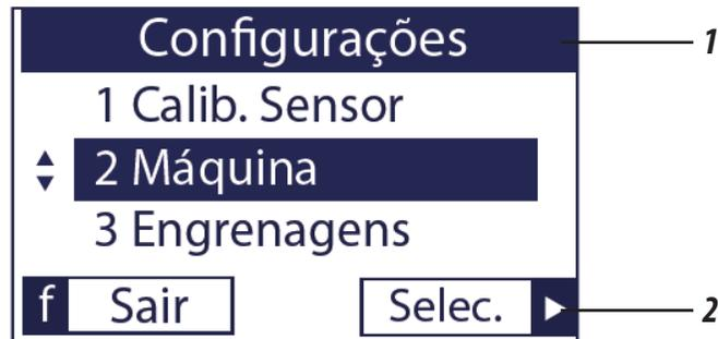
In the machine configuration (1), click on 'Select' ► (2) to inform the number of lines using the buttons ▲▼ (3).
