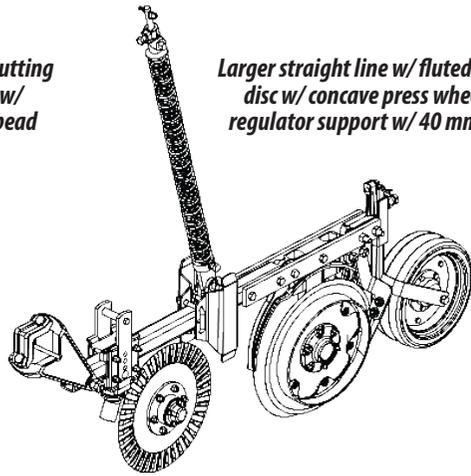
*Larger straight line w/ fluted cutting disc w/ concave press wheel w/ regulator support w/ 40 mm bead*
