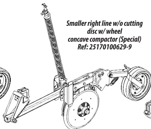
*Smaller right line w/o cutting disc w/ wheel concave compactor (Special)
