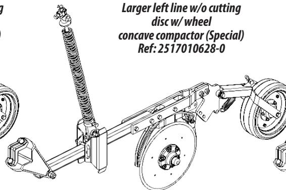
*Larger left line w/o cutting disc w/ wheel concave compactor (Special)
