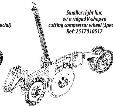
*Smaller right line w/ a ridged V-shaped cutting compressor wheel (Special)
