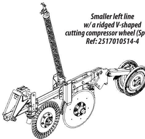
*Smaller left line w/ a ridged V-shaped cutting compressor wheel (Special)
