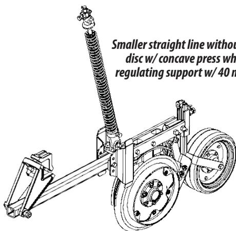
*Smaller left line w/ cutting disc w/ concave press wheel w/ regulating support w/ 40mm beading*
