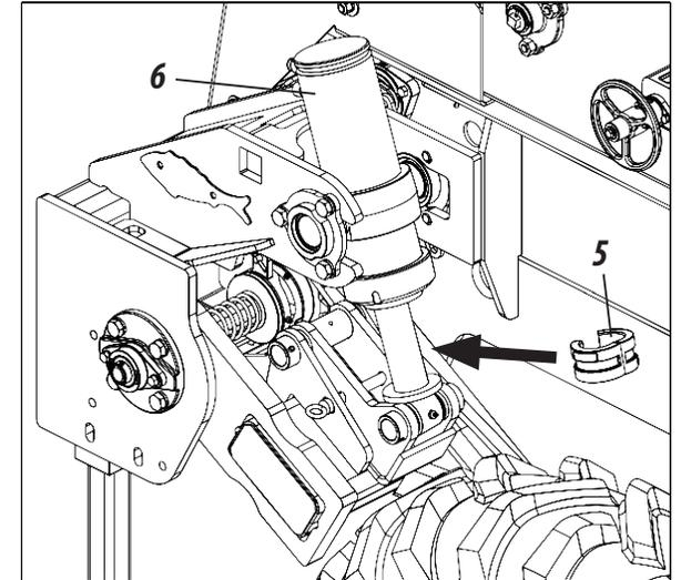
**⚠ ATTENTION** | *If necessary, also use the limiter (5) on the line cylinders (7) for depth limitation.*
