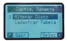
8) Then, insert the number of holes in the disc according to the crop to be worked.
