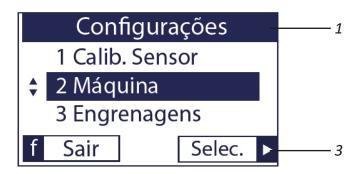
In the machine configuration (1), click on 'Select'  $\blacktriangleright$  (2) to inform the number of lines through the buttons  $\stackrel{\blacktriangle}{\blacktriangleright}$  (3).
