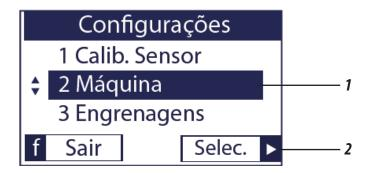
In the machine configuration (1), click on 'Select'  $\triangleright$  (2) to inform theo number of lines using the buttons  $\stackrel{\bullet}{=}$  (3).
