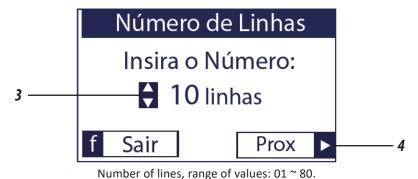
After selecting the number of lines contained in the machine, press the 'Prox'  $\triangleright$  key (4) to select the line spacing using the buttons  $\triangle$  (5).
