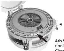
**4th Step:** Fit the adapter ring to the disc obeying the positioning.
