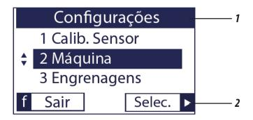
In the machine configuration (1), click on 'Select'  $\triangleright$  (2) to inform the number of lines using the buttons  $\stackrel{\triangle}{=}$  (3).
