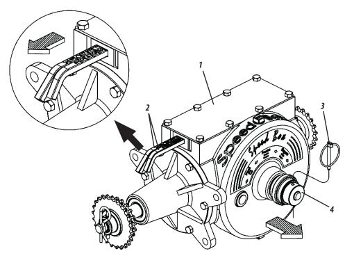
2- To move the levers, remove the lock (3), pull the handle (4), then adjust the levers as shown above. When finishing the combination, return the handle (4) and replace the lock (3).
