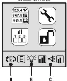
**01** - Press configure the measurement system, the display lighting the volume of the alarms.
