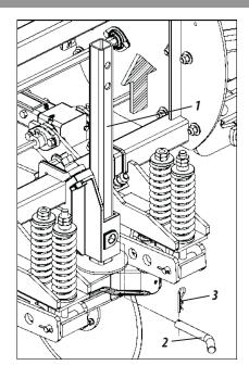
2- With the seeder down, check that it is level with respect to the ground, otherwise, level it using the header regulator (4).
