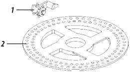
For single row discs (1), change the trigger with double rosettes to the single
