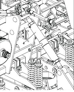
3- Then, lift the lines by fully activating the stroke of the hydraulic cylinder and place the depth gauge (5) on the cylinder rod (6).
