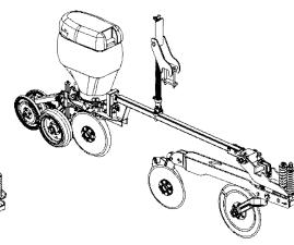
LARGER LEFT ROW WITH DOUBLE DISC WITH **GROOVED CUTTING DISC**
