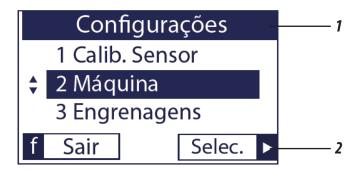
In the machine configuration (1), click on 'Select'  $\triangleright$  (2) to inform the number of lines using the buttons  $\stackrel{\triangle}{\bullet}$  (3).
