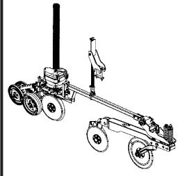
LARGER LEFT ROW WITH DOUBLE DISC WITH **GROOVED CUTTING DISC FOR 3RD DEPOSIT**
