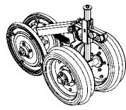
CART OF DEPTH WHEEL AND WHEEL TYPE "V" (EXCENTRIC)
