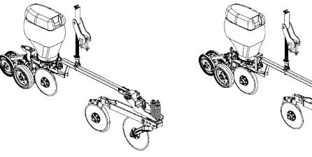
RIGHT SMALL ROW WITH LEFT LARGE ROW WITH DOUBLE DISC DOUBLE DISC
