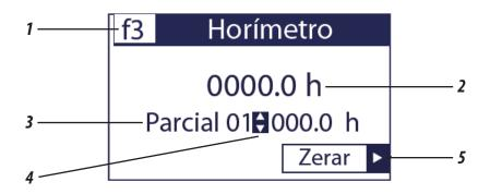
The F3 screen (1) indicates the total number of hours (2) of work with the ETD in three partials (3), which can be related to the keys  $\stackrel{\blacktriangle}{=}$  (4).
