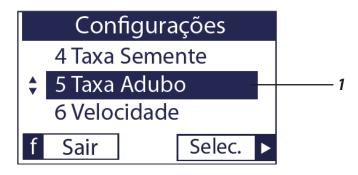
Screen F2 (1) indicates the fertilizer rate (2) in kg per hectare obtained with a specific gear ratio. Fertilizer rates are calculated according to the fertilizer calibration, the gear configuration (3) and the line spacing. The keys  $\blacktriangledown$  and  $\blacktriangle$  (4) allow the user to navigate between the rate options in Kg / ha.
