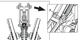
For horizontal displacement of the wheels, they were developed with eccentric bushings (5). For this adjustment, proceed as follows:
