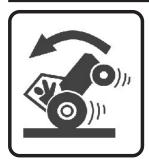
• Do not work with the tractor if the front is light. If there is a tendency to lift, add weights or ballast to the front or front wheels.
