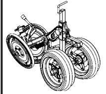
**CART OF OSCILATING DEPTH WHEEL AND COMPACTATION WHEEL TYPE "V"**
