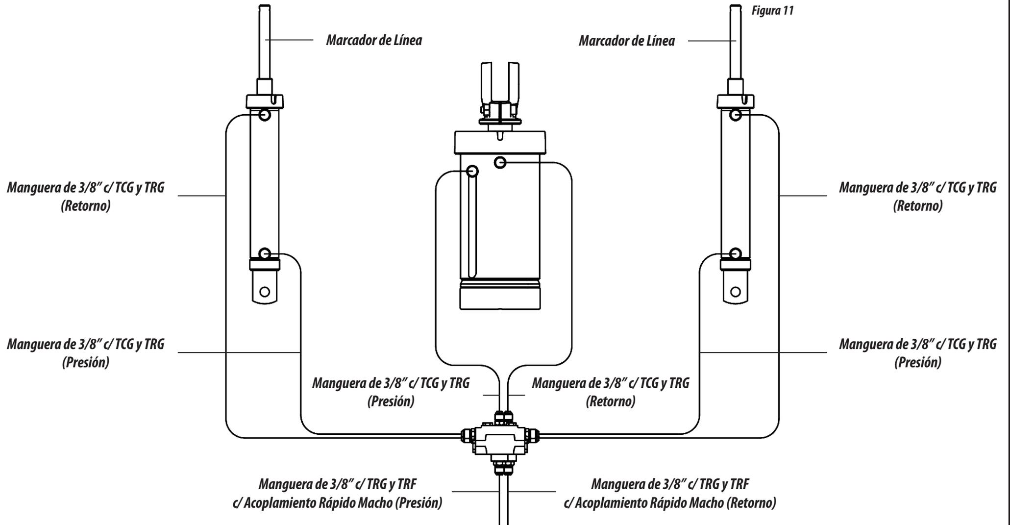
**MONTAJE DEL SISTEMA HIDRÁULICO SIN MARCADOR DE LÍNEA PPSOLO SPEED BOX TERCER DEPÓSITO 5000 Y 5500 (FIGURA 12)**
