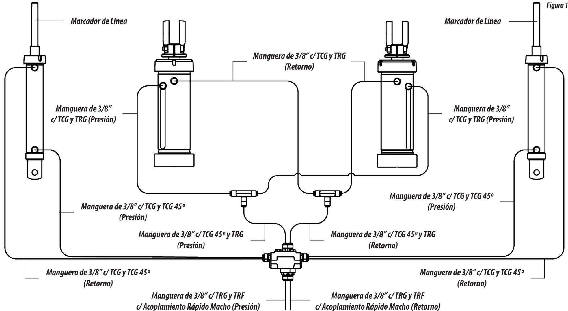
**MONTAJE DEL SISTEMA HIDRÁULICO SIN MARCADOR DE LÍNEA PPSOLO SPEED BOX TERCER DEPÓSITO 6500 Y 7500 (FIGURA 14)**
