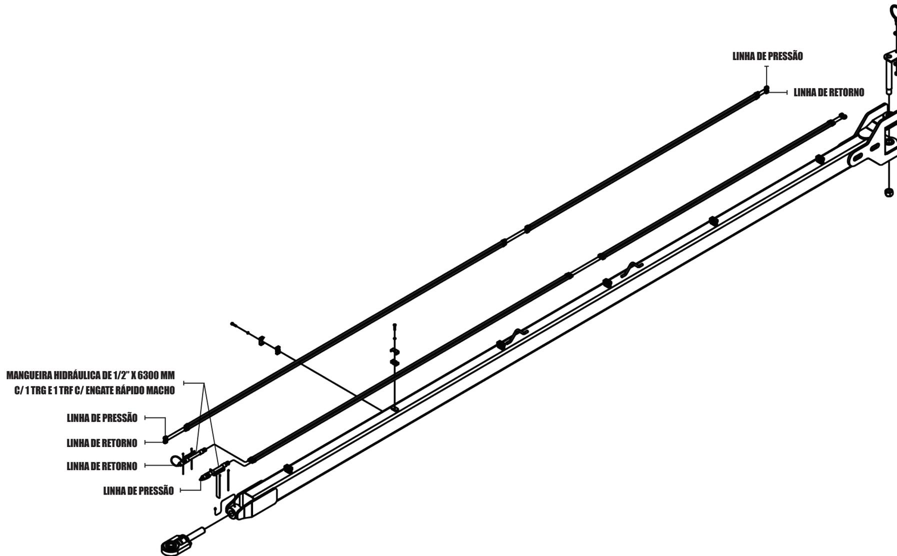
**MONTAGEM BARRA ESTABILIZADORA ESQUERDA COMPLETA PRESSÃO POSITIVA - 42 LINHAS**
