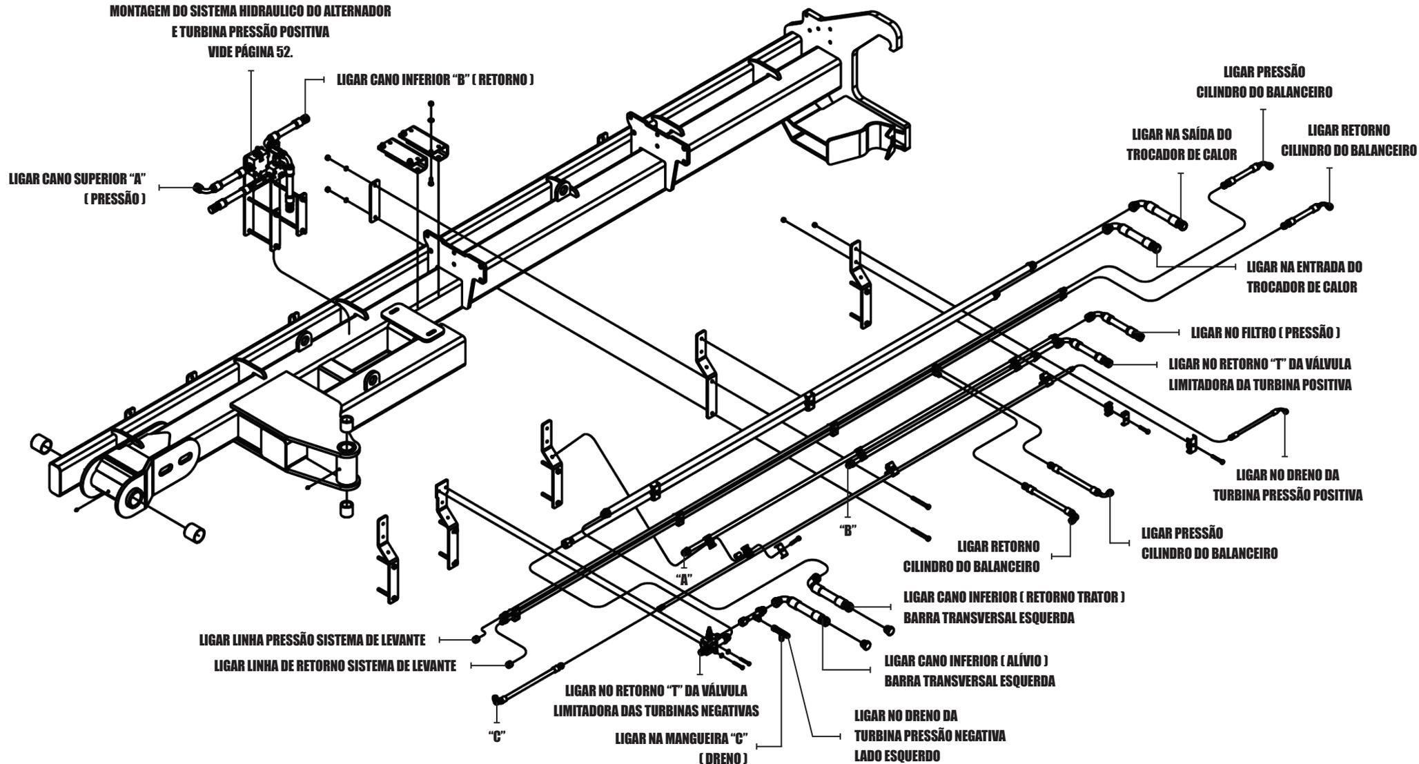
**MONTAGEM SISTEMA HIDRÁULICO DO ALTERNADOR E TURBINA POSITIVA - 34 LINHAS**
