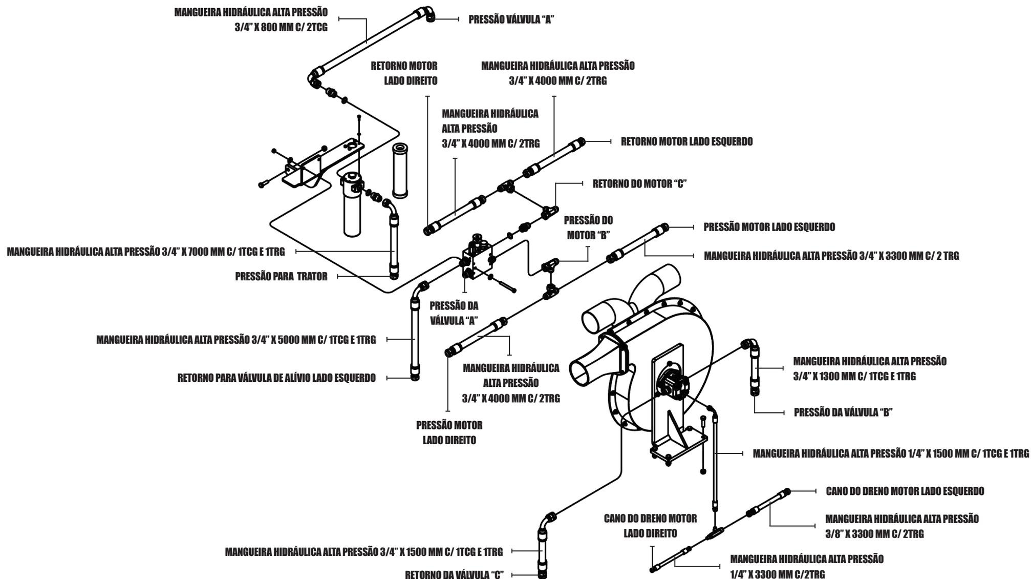
**MONTAGEM SISTEMA HIDRÁULICO C/ FLUXO CONTÍNUO C/ TURBINA MOTOR DE ENGRENAGEM PRESSÃO POSITIVA**
