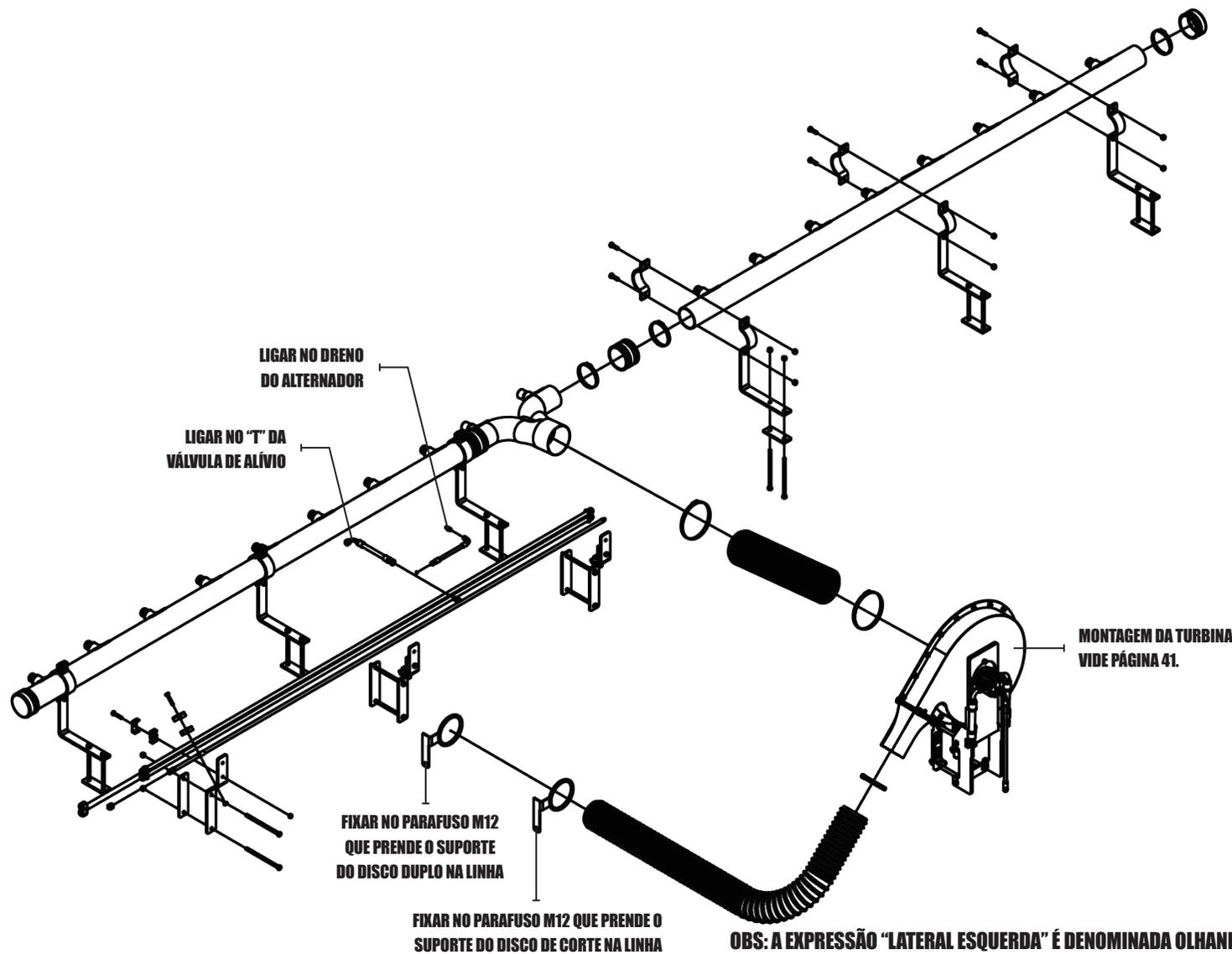
**MONTAGEM SISTEMA PNEUMÁTICO LATERAL DIREITA C/ TURBINA HIDRÁULICA FLUXO CONTÍNUO - 42 LINHAS**
