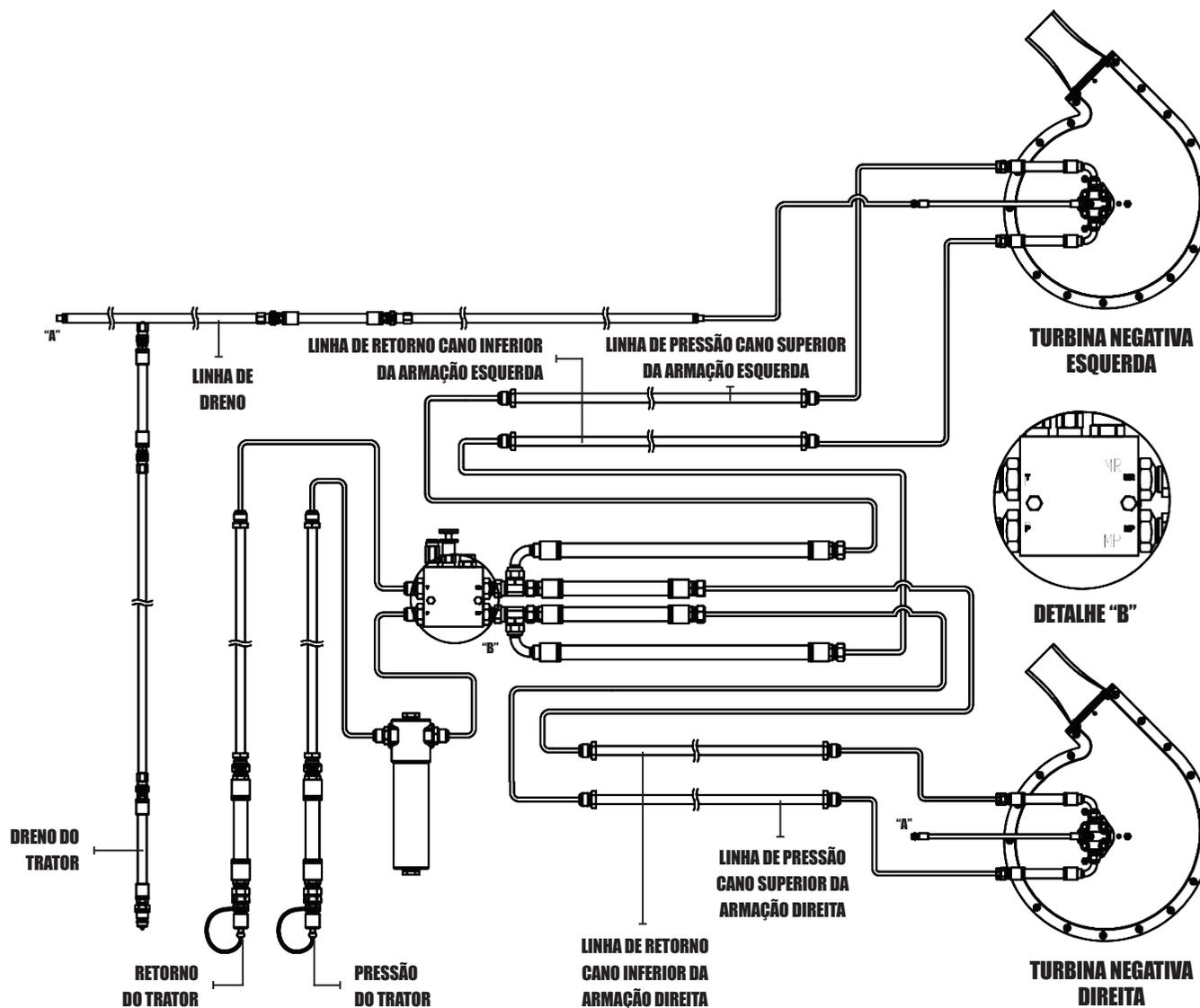
**MONTAGEM SISTEMA PNEUMÁTICO LATERAL ESQUERDA C/ TURBINA HIDRÁULICA FLUXO CONTÍNUO - 34 LINHAS**
