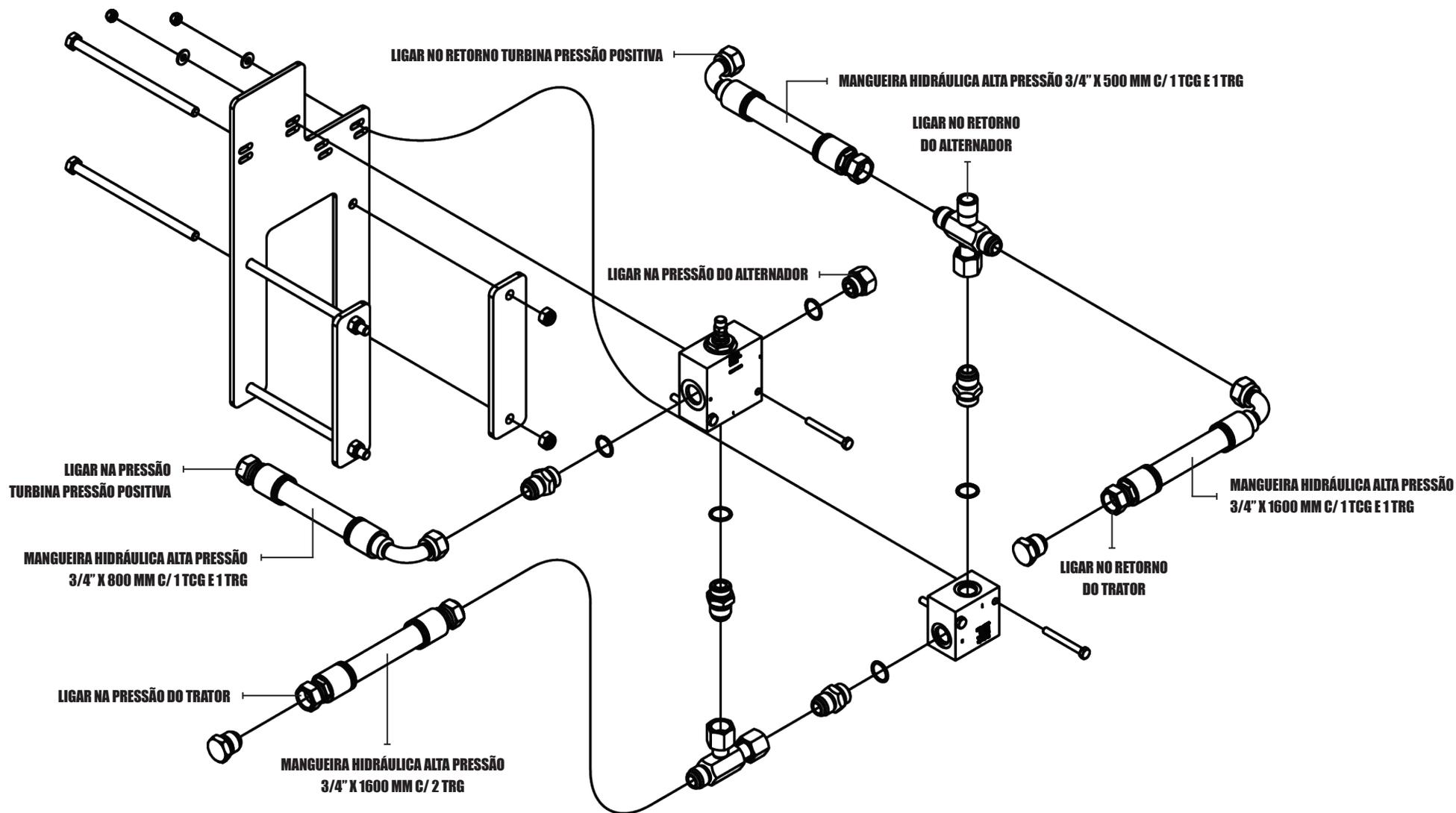
**MONTAGEM SISTEMA HIDRÁULICO DO CABEÇALHO - ACIMA DE 27 ATÉ 34 LINHAS**
