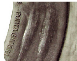
Very evident wear in this area that can cause doubles (two seeds in the same hole of the disk).
